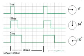
Similarly, 2.0ms pulse will make a clock-turn to  $180^{\circ}$  and 1ms pulse will make an anti clock-turn to  $0^{\circ}$ .
